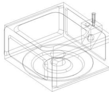
Fig 1. Geometric model of the microwave oven
