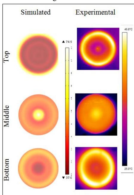
Fig 2. Temperature (°C) profiles of simulated and experimental gel planes
